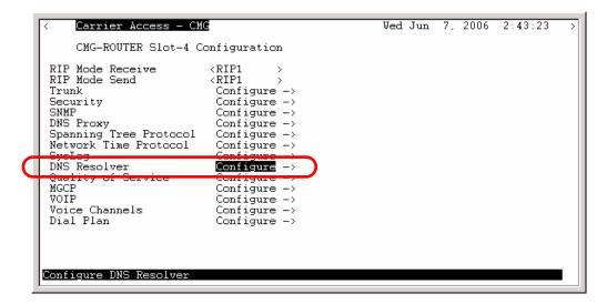
To enable DNS Resolver, scroll <Disabled> to <Enable>, with the [SPACEBAR], select [ENTER].
